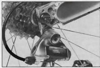
Hate, hatred, hateful: For some reason Crosstrac put difficult-to-use rear entry dropouts on the Sonoma's swingarm. To make matters worse, the axle nuts are recessed into the machined axle plate. Safety dropouts on the rear? Give us a break—or a hammer.
