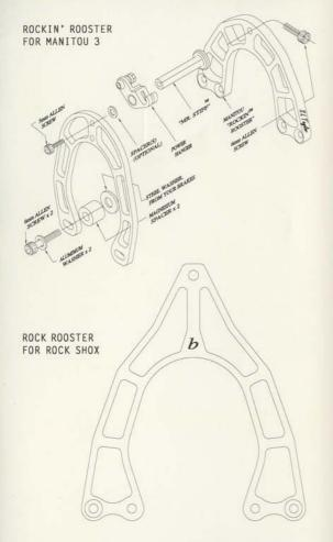
THE CNC MACHINED 7075-T651 ALUMINUM ROCK ROOSTER HELPS ELIMINATE THE LATERAL FLEX INHERENT IN SUSPENSION FORKS. NEW THIS YEAR IS THE ROCKIN' ROOSTER FOR ROCK SHOX AND THE MANITOU 3. MORE POWERFUL AND TRICK THAN THE STANDARD ROOSTER, THE ROCKIN' ROOSTER PACKAGE COMES COMPLETE WITH A ROOSTER, A CANTILEVER BOOSTER, MR. STIFF, A SUNTOUR POWER HANGER, MOUNTING HARDWARE, AND A COMPREHENSIVE SET OF INSTRUCTIONS.
