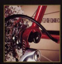
Breeze-In<sup>TM</sup> dropouts provide light, rigid support, with half the weight and twice the stiffness of standard dropouts. They maximize the efficient power transmission of the chainstays and bolster the rear derailleur for better shifting. Ramped faces smoothly guide hub into frame.
