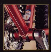
Steel tubing is precisely butted to add strength and pare weight. Seat tube is flared and elliptical at bottom bracket, forming a larger cross-section that resists pedaling-induced lateral flex. Shimano's Torlon cable guides fight friction for smooth shifting even when bone-dry.
