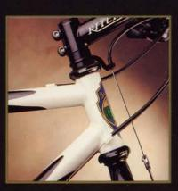
Wide spacing of top and down tubes gives greatest frame strength per head tube length. Head tube bottom is externally butted. Shift housing stops are brazed onto head tube to avoid heat stress to down tube and are positioned for maximum brakecable clearance. New AheadSet system gives stronger, stiffer and lighter stem connection.
