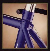
Bulge-butted seat tube is stronger and straighter than common sleeved type. New "snake tube" brake slider blazes a light and efficient path for the rear brake cable. Placing QR binder slot on front of seat tube reduces inflow of water and grime off rear wheel. Scalloped seat binder (not seen in this view) prunes weight.
