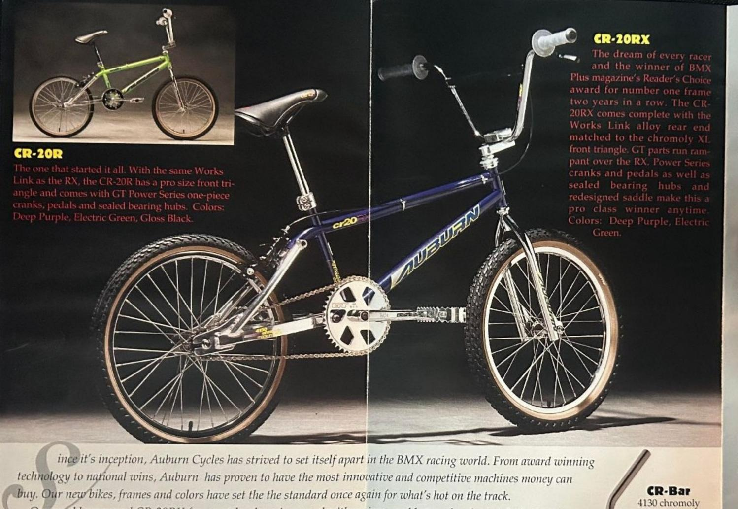
Our world renowned CR-20RX frame set has been improved with an increased bottom bracket height for better ground clearance, and bigger down tubes specially sized to increase strength yet retain their light weight. Also, we have a new mini frame, the MR-20RX, which is a smaller version of the popular JR-20RX. And Cruiser fans
