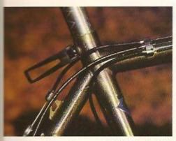
The angles on the test bike come out at 71.5° head and 74° seat; so fitting even a shortleg suspension fork would lay back the angles by at least a degree...
