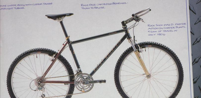
CHAINSTAYS - ONLY \$18mm. GREAT FOR ABSORBING SHOCK; BETTER TIRE CLEARANCE, AND A BUILT-IN CHAIN-SUCK PROTECTOR.
