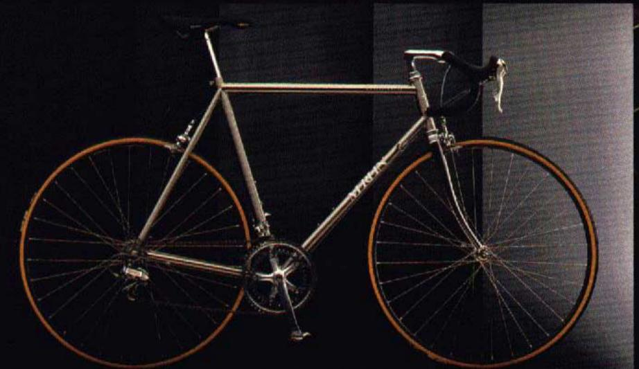
optimum distribution of stress loads, better management of unwanted flex, and longer frame life. The top tube, down tube, head tube and chainstays are all double-butted, while the seat tube is single-butted at the bottom bracket (and reinforced with an integral sleeve at the seat collar). In this way, extraordinary strength is maintained at the welds, while a controlled amount of resiliency is permitted in the thinner center spans to deliver supple wheel control and matchless comfort.
