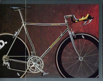
Tachyon is defined as a hypothetical sub-atomic particle that travels greater than the speed of light and possesses infinite energy. Since its introduction, the design of the **Litespeed Tachyon** has set the standard for aerodynamics and rider positioning. Custom aero-oval tubing and enhanced aero-positioning work together to reduce frontal area which in turn greatly lessens wind resistance. However, the Tachyon does not sacrifice comfort and stability for aerodynamics.
