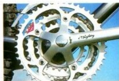
The Sugino Mighty crankset weighs less than XTR, but shifting isn't as smooth.
