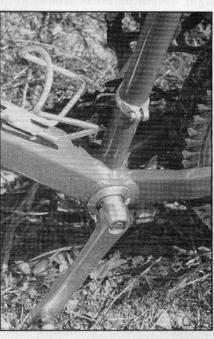
The CQP precision sealed bottom bracket and top pull derailleur come standard with the F-26. The only tube on the bike that isn't tapered rectangular is the seat tube as it is a non-stress bearing tube.
