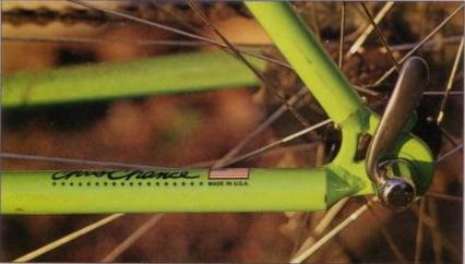
The non-tapered chainstays provide key stiffness to the rear triangle, making the Buck Shaver an exceptional bike for climbing.
