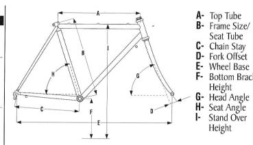
Note: Frame Size/Seat Tube dimensions are center-to-top on all mountain and cross models, and center-to-center on all road models.
