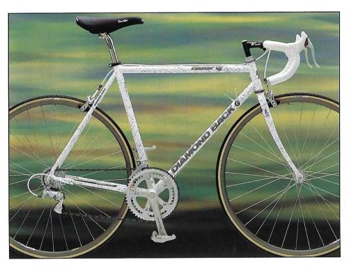
The bike's a beauty, sure, but that's not why we TIGweld by hand its oversize, thinwall, thermally enhanced True Temper RC2 chromoly tubing. We do it to give you pulse-pounding acceleration, whether you're crossing the finish line with your hands in the air or topping out the toughest climb on a ride.
