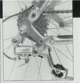
Horst link: Perhaps the most imitated element of a Horst Leitner suspension design is the "Horst Link." By pivoting the seat and chainstays at the rear dropout, the link eliminates the torque forces of braking and pedaling from the suspension system.
