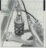
AMP shock: The rear triangle gets its rigidity from the wide mounting and multiple pivots of the machined aluminum Aarm shock linkage. The shock is an oil-damped, thru-shaft shock that is operated by the straight-rate suspension linkage. The seatpost QR is machined out of a solid block of 6061. Very trick.
