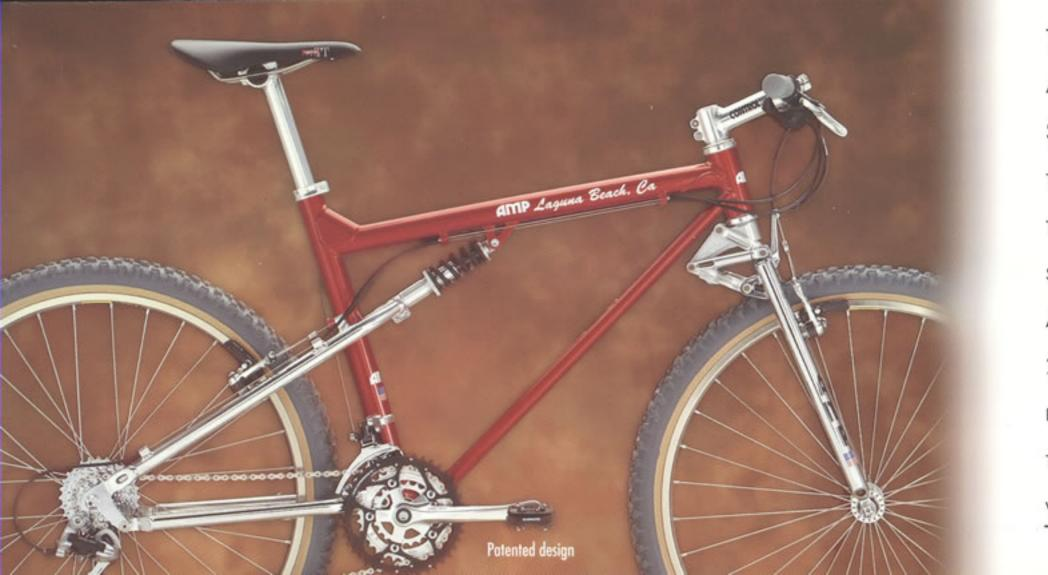
THE PERFECT COMPLIMENT TO THE AMP FORK IS THE AMP FULL SUSPENSION FRAME, UTILIZING THE SAME THRU-SHAFT SHOCK TECHNOLOGY AND CHROME SILICON SPRING AS THE FORK, THE AMP FRAME PROVIDES A SUPPLE 2.75" OF TRAVEL. THE STRUT TYPE REAR SHOCKSTAY IS JOINED TO THE SWINGARM WITH THE MOST WIDELY USED AMP
