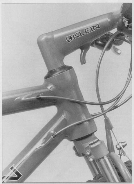
As big as it gets: You won't find another headset system on the market that is bigger than Klein's. Originally designed to accommodate the oversized aluminum steerer tube of the Klein aluminum fork, the head tube accommodates the Rock Shox steerer tube by using a steel sleeve. The Rock Shox are custom-painted to match the frame.
