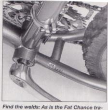
dition, craftsmanship is first-rate and is exemplified by some of the prettiest welds in the industry. Asymmetrical chainstays help maximize chainring clearance.
