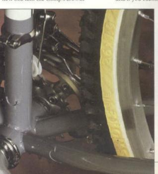
If you want an alternate fork, Bontrager will sell you a Race Lite with a RockShox. Of course, it's not that simple: The RockShox-endowed OR Race frame is tailored for the marriage. To compensate for the extra front-end lift of the suspension fork, Bontrager varies the geometry to arrive at 71/74-degree angles. And he shortens the top tubes by a half-centimeter to get more rider weight on the front wheel—a reasonable goal when a shock-absorbing fork is there too.
