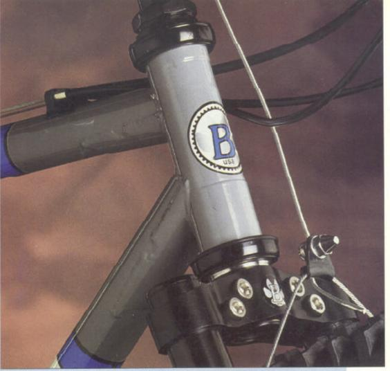
The Race Lite's quest for strength avoids oversize dimensions. Even with the requisite reinforcements, the frame is very light, weighing just over four pounds.
