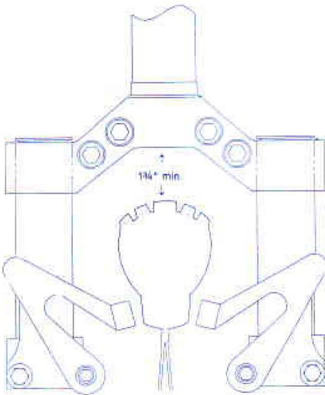
**WARNING:** Do not raise or lower the fork tubes in the crown. This could cause lack of proper tire clearance when the fork compresses or reduce the amount of fork leg engagement at the crown. Either case constitutes an unsafe condition.
