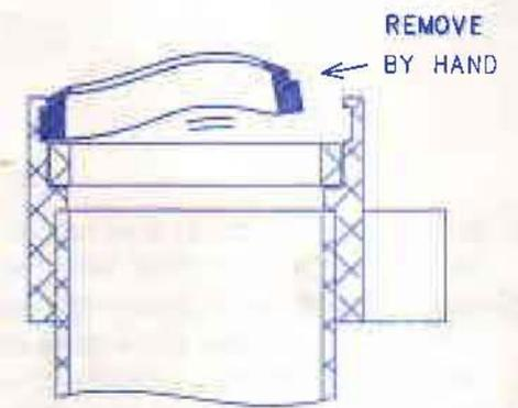
**Removal of Compression Rubber and Lower Bushing**
