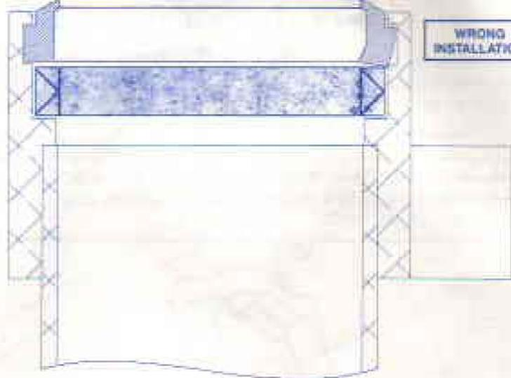
This illustration shows correct seal installation at the left, and incorrect installation at the right. Use a finger to run around the seal once installed to confirm that seal is properly installed and fully seated at all points.
