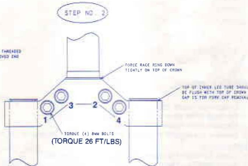
**WARNING: Do not raise or lower the fork tubes in the crown. This could cause lack of proper tire clearance when the fork compresses or reduce the amount of fork leg engagement at the crown. Either case constitutes an unsafe condition.**
