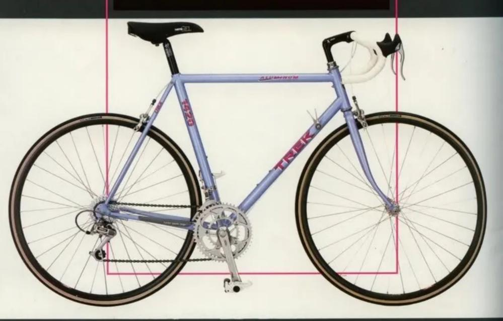
The 1200 is Trek's most popular aluminum road bicycle. It features a double butted, bonded aluminum construction which results in a strong, stiff, but very light frame. It is equipped with a Shimano RX-100 SIS drive train and Matrix 1SO-C II rims. This is a bicycle that delivers the acceleration, speed, and durability needed for riding at your best.
