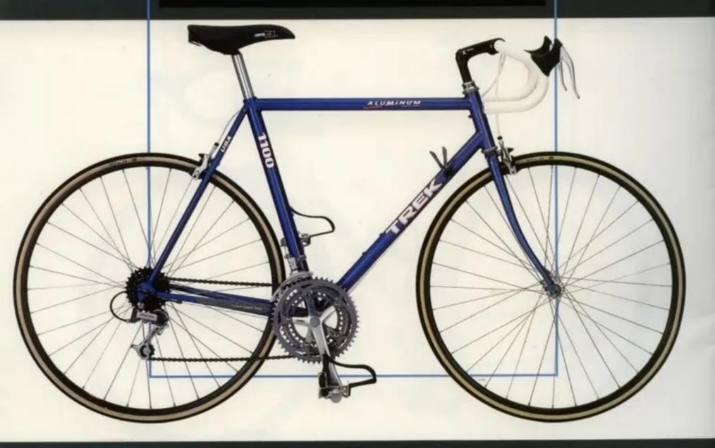
The 1000 offers aluminum performance at a value price. The frame consists of double butted aluminum tubes which are bonded to our exclusive investment cast lugs. This construction results in a light, strong, and precisely aligned frame.
