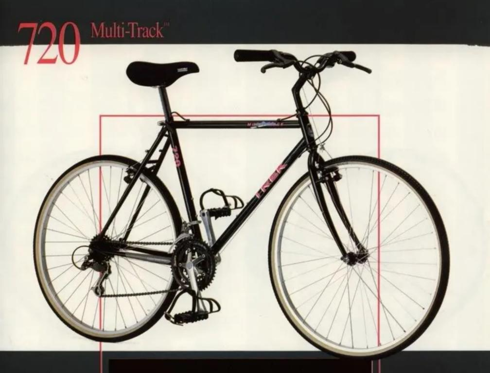
Comfort was the main concern when designing the 720. Its geometry and handlebars create a riding position that allows the cyclist to sit upright for increased comfort and reduced fatigue. The SunTour XCT components mean effortless shifting which is important for an enjoyable ride. The Matrix Multi-Track tires are smooth rollers that make hill climbing much easier and also lessen the effort needed to maintain speed on the flats. When you are pedaling
