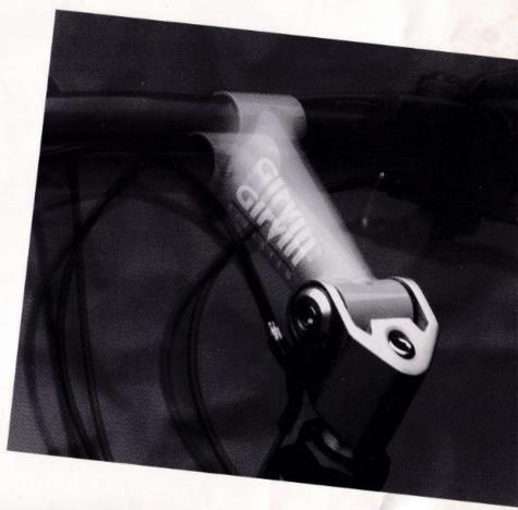
When riding over bumpy terrain, forces are created which act to slow forward motion (borizontal component) and transmit impact (vertical component) to the rider. Pro-Flex suspensions, with their advanced elastomer disc "springs", reduce total bump forces for a faster, more controlled ride.
