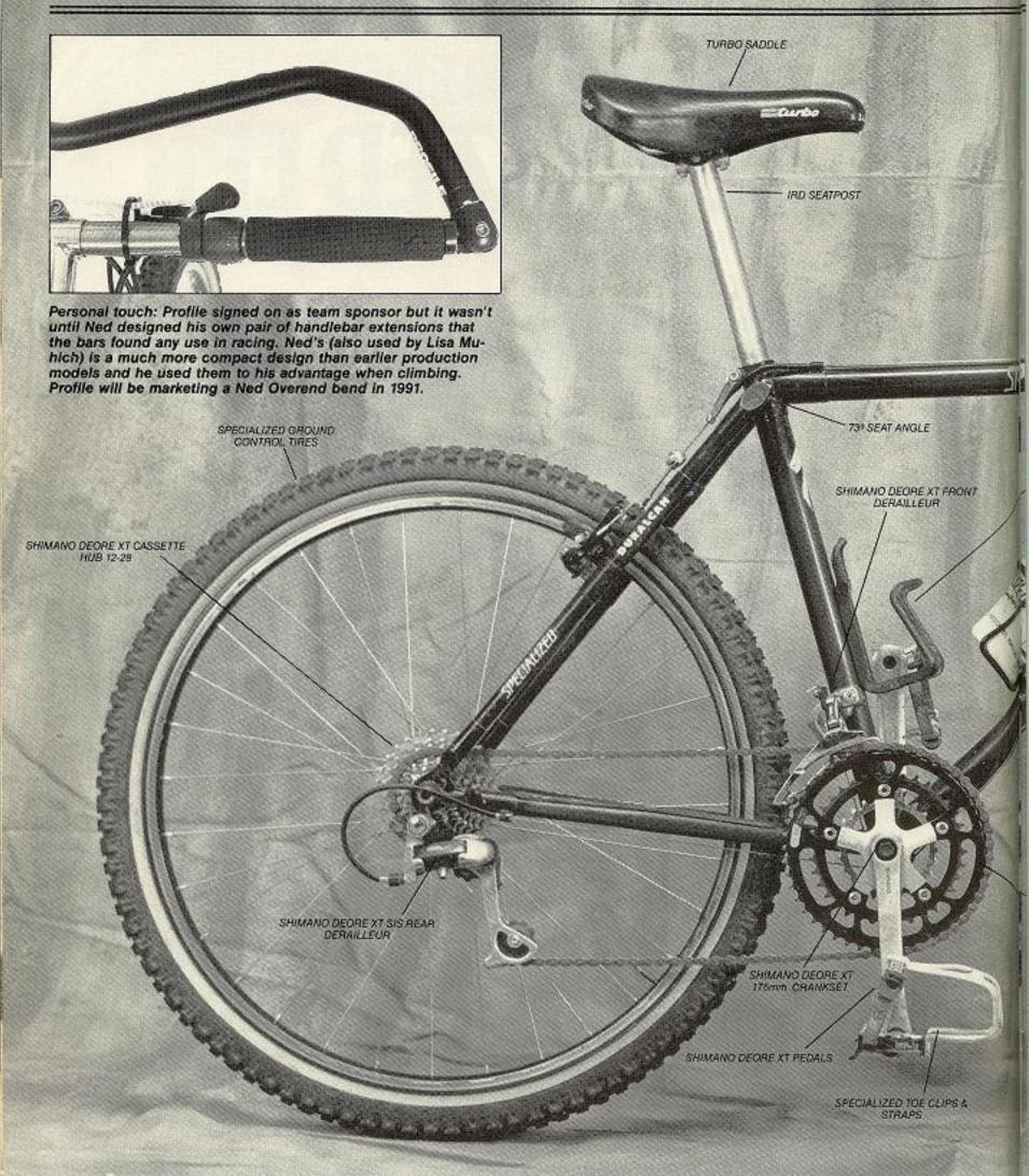
middle ring, but Shimano didn't make an SG version this year and they really work sweet so I switched to the 36. In the rear I used a 13-30 Hyperglide combination. At Durango it was threatening to rain, and I figured I'd need the extra gears if it got wet.
