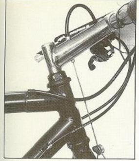
Not a flaw found: Craftsmanship on Ned's blke is first-rate. Unlike other brands, Specialized downplays the visible aspects of the carbon tubes and titanium lugs to give the bike a very plain-wrap appearance. To soften up the ride when he's not using Rock Shox and to save more weight, Ned uses a titanium stem and handlebar combination, compliments of Litespeed.
