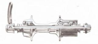
The Shimano freehub combines the rear hub and freewheel mechanism into a stronger one-piece unit. The advantages of freehub design are more advantageous placement of spoke flanges, placement of the hub bearings closer to the dropouts, and a stronger rear frame triangle to enhance power transfer efficiency.
