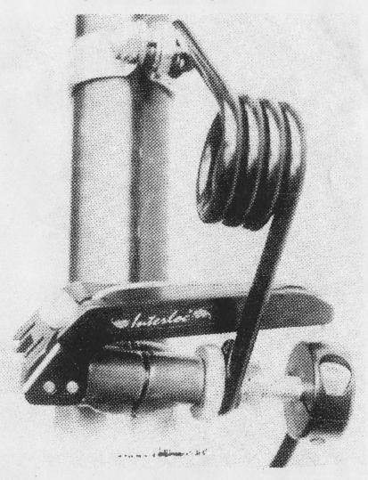
For those of you who would like to adjust your seat height without fumbling under your seat, we at Interloc have developed a powerful little clamp that can be operated with a shift lever on your handlebar. It is used in conjunction with a "Hite Rite" spring.
