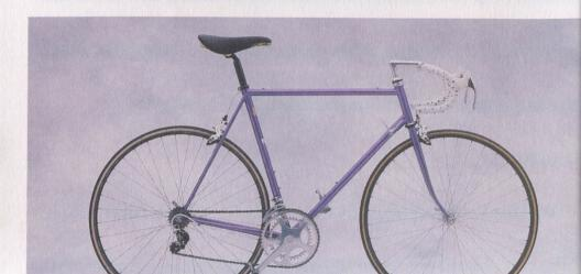
To remove, just unscrew. Like the Wicked, the Team has a 71 degree head tube angle and a 72 degree seat tube angle. The fork is our newest design, light weight (1 pound, 12 oz), plenty of clearance, utilizing oversized butted straight blades for maximum shock absorption and 1.5" rake for quick handling without compromise. Both front and rearwheel clearance is ample for the new 2.5" tire.
