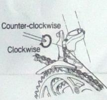
The high gear adjusting screw is used to adjust the position of the front derailleur. If the clearance between the chain and the inner cage is too much, turn the adjusting screw counter-clockwise. If the chain countacts the inner cage, turn the adjusting screw clockwise, but not allowing lever A to return to the center position (Fig. 3-K)
