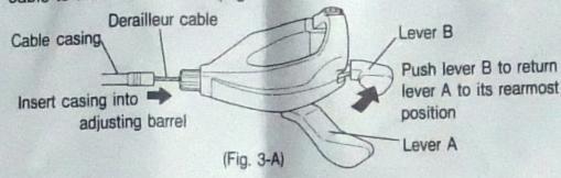
With the chain on the smallest chainring, turn the crank slowly while pushing lever A to the first click position, shifting the chain onto the second smallest freewheel cog.
