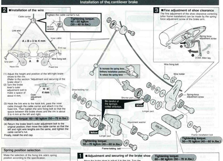
Move the brake shoe to adjust it to the rim. Turn the adjustment washer and adjust so that the rim surface and shoe surface are as shown in the figure. After the
