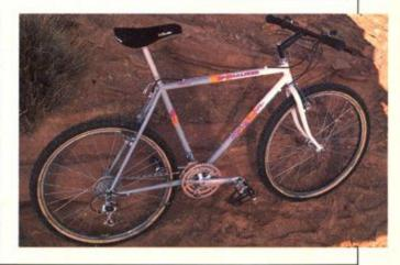
inches of fork rake. The seat-tube angle is 73 degrees, chainstay length is  $16^{7/8}$  inches, and wheelbase is  $41^{5/8}$  inches. Stem extension and rise felt right.
