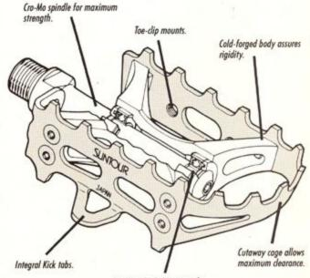
Precision Sealed bearings for low friction, high durability.
