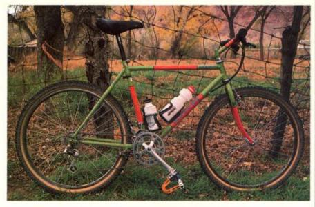
ment-cast to resist the stress of opening and closing the quick release. The lug features a rear-facing tab for mounting a Hite-Rite saddle height adjuster, and forward-facing ears for a more accessible quick-release lever. The head tube, another high-stress area, is strengthened top and bottom with external reinforcing rings cut to mimic fancy sculpted lugs. The head tube and the seat lug are also adorned with badges of Lindsay's goat-head logo.
