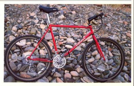
large, slotted cable stops, a solid rear brake bridge, toe clips and straps, and bosses for two water bottle cages located low enough to permit use of a shoulder strap. Tires are Ritchey Force 2.0s mounted on Araya RM-20 rims. The drivetrain has that ubiquitous Shimano combination of 12-28T Hyperglide cassette freehub with 28/38/48T Biopace chainrings-gearing that's too high for most riders.
