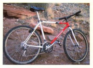
Ritchey also supplied his 435-gram Vantage hard-anodized rims (32-hole, of course) and dirt-hungry Force 1.9 tires. The rims are laced with Wheelsmith stainless steel spokes to SunTour's XC-9000 hubset, including its new 7-speed cassette freehub.
