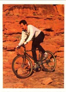
inch top tube (on our 19-inch test bike) combined with a 11.5-cm, medium-rise chrome-moly stem to put the rider in a powerful yet well-balanced position for the best mix of climbing, descending, and cornering control. We rode primarily on snow-covered roads and trails and
