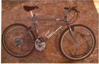
are mounts for two water bottle cages. Cable stops are large and slotted for easy maintenance. Tires are Ritchev Force 2.0s mounted on Araya RX-7 rims with Mountain LX quick release hubs.
