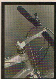
Solid billet: A block of aluminum billet is machined to build a finely crafted solid stem. The complete system is very similar to the successful designs used in BMX racing for the last ten years. Excellent workmanship and lots of extra work for Manitou.
