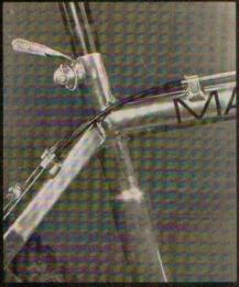
Doppleganger: Manitou has a seat tube that uses two different-diameter aluminum tubes. From the bottom bracket up, a 1.50" tube is welded to a 1.25" tube. The advantages are tight clearances for the seatpost and extra beef for the bottom bracket.
