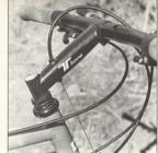
Long John: The long Tioga T-bone stem gives the Ascent a tendency to oversteer the front end at speed. One noticeable advantage to straight blade forks is the distance that the front brake cable clears the headset by
