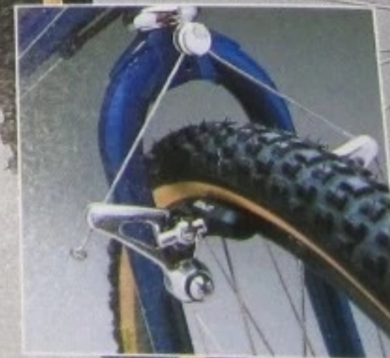
New Deore-XT cantilevers with "No Pinch Cable Carrier," Specialized lugged uni-crown fork
