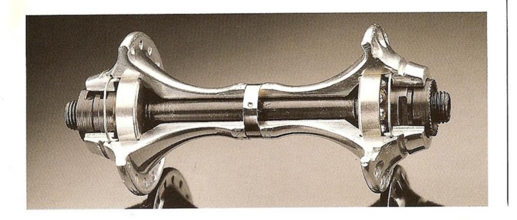
The cone, cup, ball mechanism, unlike the scales bearing system allows for fine adjustment (by means of Campagnolo wrenches 7130010). Once again, 02-ZPT grease is recommended for lubrication.
