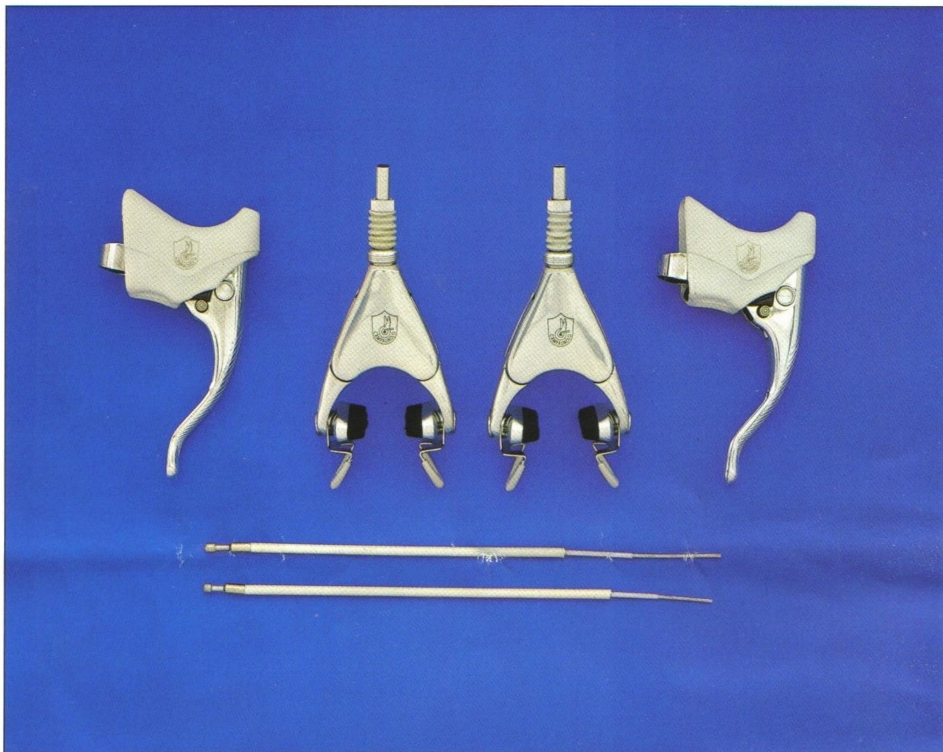
The RECORD group is equipped with a center pull brake with an articulated parallelogram.
