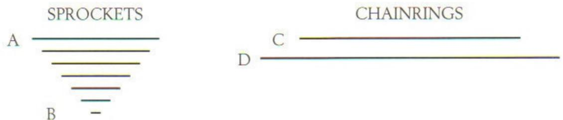
$$\text{Gear change capacity} = (D + A) - (C + B) = 30$$
