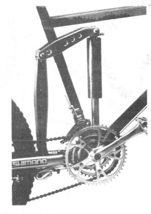
This Exclusive C-Link rear suspension's rising-rate design can handle almost any terrain.
