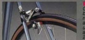
Dia-Compe's new GX500N professional brakeset with quick release (dark anodized). Araya 20A ultra-narrow dark anodized clincher rims 27x1, 100 psi tires.
