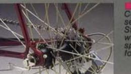
Suzue dark anodized Competition hubs with sealed system. Stainless steel spokes with black chrome spoke nipples. Shimano lorged dropouts.
