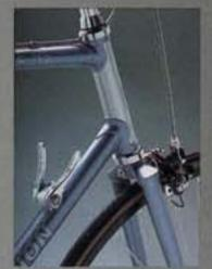
Lightweight, gracefully styled fork crown with internally mounted brake bolt. Tange Aero headset with precision bearings. SunTour's top mounted, self-adjusting levers. Brazed-on cable guides
