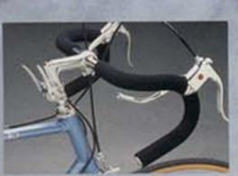
SR aluminum stem. Cushion grip handlebar covers. Safety brake levers. Aluminum stem mounted shift levers.
