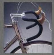
SR cold-forged aluminum stem and bar. Gran Compe cantilever brakes with Centurion exclusive brake pad design. Professional brake levers with gum hoods. SunTour Top Mount self-adjusting shift levers.
