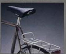
Centurion heliarc-welded rack attaches neatly to seat stay bosses. Vetta Italian anatomic seat with genuine leather cover. SR Laprade aluminum seat post.
