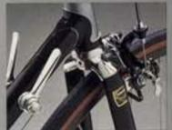
Investment cast aerodynamic integral fork crown. Recessed brake mounting bolt. Compact, thin-walled (1mm) hi-tension lugs. SunTour Superbe Pro levers mounted on brazed-on bosses.
