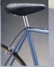
Dia-Compe aluminum brakes. Padded seat. Brazed-on cable guides.
