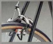
Dia Compe new Gran Compe professional brakeset (short reach) with new improved quick release mechanism. Exclusive Centurion curved brake bridge with integral mounting bolt.
