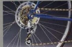
SunTour ARX wide ratio aluminum derailleur and Pro Compe 14-30T 6 speed gold freewheel. DID gold and black chain with bevelled plates for smooth shifting. Araya narrow aluminum anodized rims. Forged anodized rims. Forged frame dropouts.
