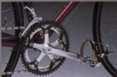
Shimano New 600EX: cold-forged aluminum crankset; aerodynamic platform pedals; and front derailleur. Araya 20A ultra narrow dark anodized rims. Toe clips and straps included.
