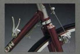
Internal electrical wiring system supplies headlamp from stay-mount dynamo (not included). Dia Compe 960 cantilever brakes with hooded levers. SunTour Top Mount self-adjusting shift levers
