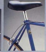
Dia-Compe aluminum brakes. Selle Royal anatomic aluminum hub with seat. Brazed-on sealed mechanism. cable guides.
