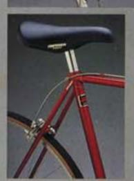
Wetta anatomic seat made in Italy, Stainless steel seat post. Brazedon cable guides,
