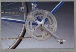
Sugino RT full aluminum 40/52T crankset with chain-guard. Will accept sprockets from 34 through 54T. SR SP 150 aluminum pedals. SunTour ARX widerange front derailleur. Brazed-on water bottle bosses. bosses.
