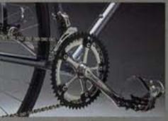
Sugino Astron cold-forged crankset with dark anodized outer ring, SunTour Cyclone MK II derailleurs, SR Sil-Star pedal, Toe clips and straps included.
