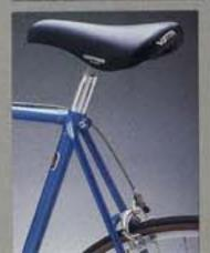
Vetta anatomic seat made in Italy. SR Laprade aluminum seat post. Dia Compe N500Q brake. Exclusive Centurion curved brake bridge with recessed bolt.
