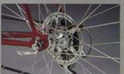
Quick release rear wheel. Suzue aluminum hub with sealed
