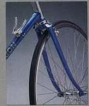
Graceful Centurion forged crown with recessed center bolt. Recessed SunTour Top Mount self-adjusting shift levers. Suzue aluminum quick release hub with sealed system. Stainless steel spokes. Araya narrow aluminum rims.
