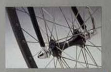
Suzue competition sealed bearing hubs. Stainless steel butted spokes. Araya 20A ultra narrow rims. Chrome plated fork tip.
