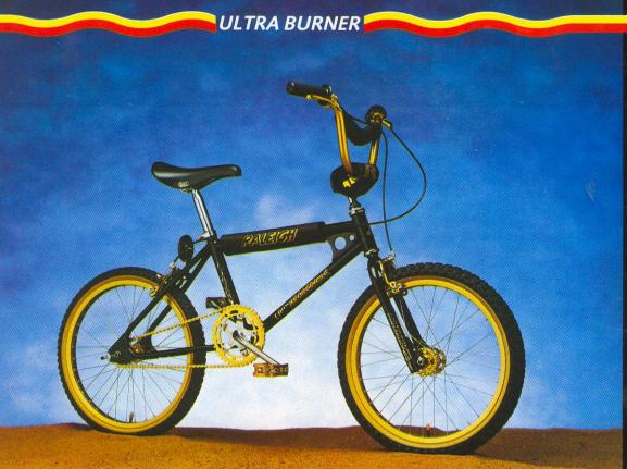
Another thoroughbred built around a frame and fork made from controlled carbon steel tubing developed by Raleigh-Carbospec 23. This machine has a full race proven spec with such unbeatable components as Suntour four-bolt stem with Cro-moly tube, Suntour large flange hubs with Cro-moly axles, Sugino one piece, polished, chrome plated Cro-moly crank, Araya 7X rims and Dia Compe brakes. More up-todate style with Raleigh's own lightweight velcro pads and an aerodynamic saddle.
