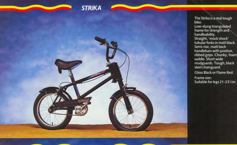
The Strika is a real tough Low-slung triangulated frame for strength and handleability. Straight, 'mock shock' tubular forks in matt black. Semi-rise, matt back handlebars with positive, ribbed grips. Chunky, foam saddle. Short wide mudguards. Tough, black
