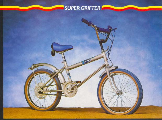
The Super Grifters are all bike for boys who are all boy. They're top of the Grifter class and a serious proposition. Double-clamp stems. Sprung and padded saddle. Big, big-clearance rear mudguard. Drilled chainwheel disc. Three-speed gears with click-stop, twist-grip control. Rough-stuff tread, gum-wall tyres. Rubber reflector pedals.
