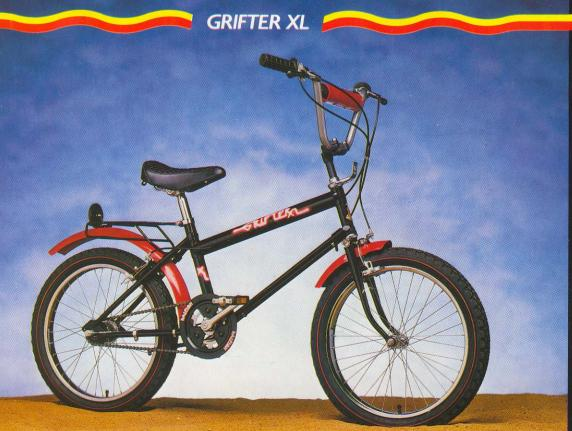
The Grifter plus. Plus a sturdy, frame-attached rear carrier. Plus satin chrome handlebars. Plus a red crash-pad on the handlebar cross-tie. Plus Redline tyres. Plus narrow, quilted saddle and fourbolt stem head.
