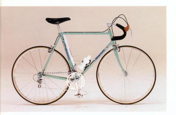
Quick-handling and responsive, the Professional is happy on a twisting country road or racing Criteriums. Tight geometry and completely double-butted Chrome-Moly frame combine with Sugino SuperMighty crankset, Suntour Superbe Pro derailleurs, New Winner 6-speed freewheel, Selle Italia Aero II saddle, and Panaracer 270 gram tubular tires. To give you professional performance. Colors: Celeste, Black
