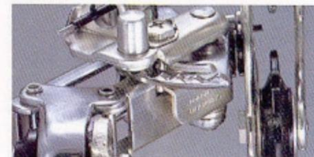
Positive Indexing Mechanism on Positron-II Rear Derailleur
