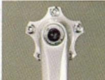
Long service life is assured by 5 pins with fixed position nuts.
