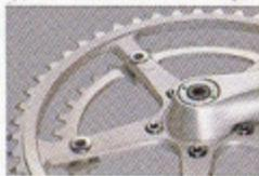
Forged outer sprocket with aerodynamic styling.
