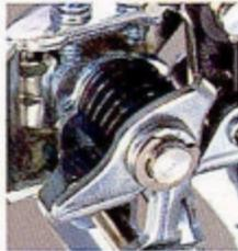
Pre-Select Mechanism on Positron Front Derailleur
