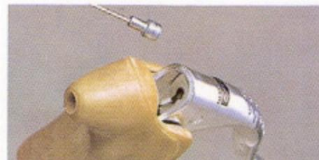
One-step cable attachment mechanism (Shimano 600EX Brake Lever).
