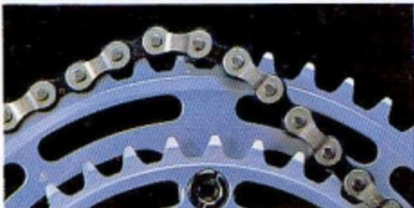
Rear side view of chain moving to low gear off W cut teeth.
