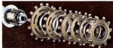
Spline-type cassette gear of Dura-Ace EX Freehub.
