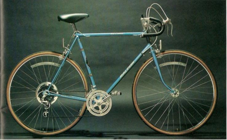
Frame: Size: Gents: 19¾", 21½", 23½", 25". Ladies Mixte: 19½", 21½". Constructed with Raleigh lightweight lugs & Raleigh 20-30 high carbon steel tube. Features brazed-on cable eyes, guides, downtube stop &
