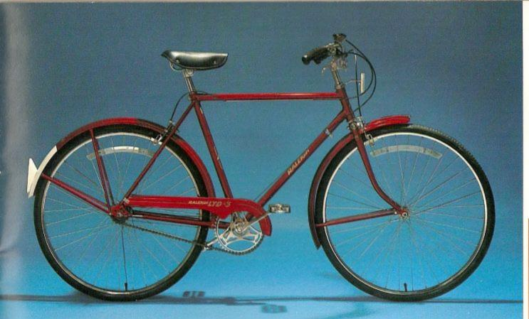
The Raleigh LTD is built to the same exacting standards that have made Raleigh the foremost name in cycling throughout the world. The LTD features fully lugged frame construction and famous Raleigh tubular fork and crown which provides great strength ①. The LTD is available with either Sturmey Archer 3-speed AW hubs with trigger control or coaster foot brake hub. The new chainguard provides extra protection and is attached with brazed mounts for secure rattle-free use ②.
