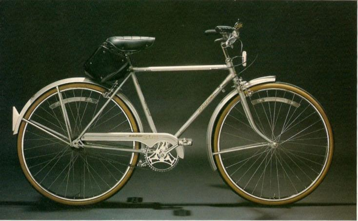
A classic in its own time with a reputation for quality, comfort and reliability that spans the globe, the Raleigh Sports is constructed of 20-30 high carbon steel tubing with Raleigh feature cut lugs. Brakes are the new Raleigh/Weinmann model fitted with lightweight alloy levers 1. Saddle is the new Brooks vinyl seat with sprung frame to provide riding comfort, plus saddle bag for carrying convenience (2).
