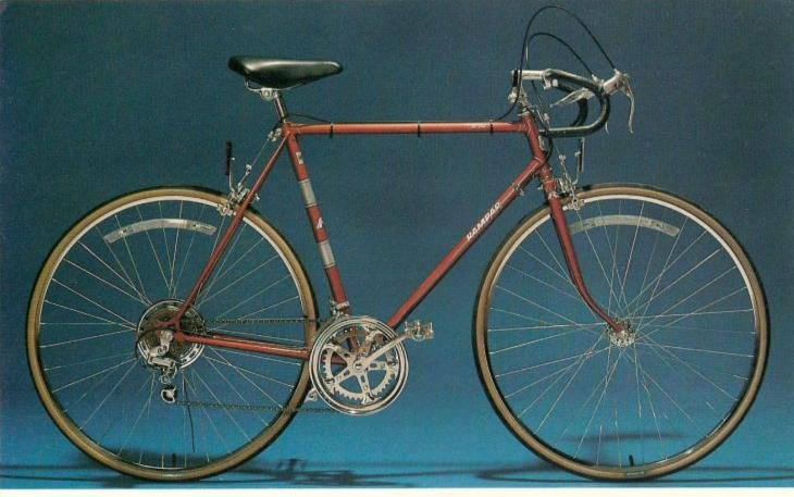
Frame: Size: Gents: 19%", 21½", 23", 25". Ladies: 19%", 21½". Constructed with custom cut lugs & high carbon steel tube. Features brazed-on cable eyes & downtube stop.
