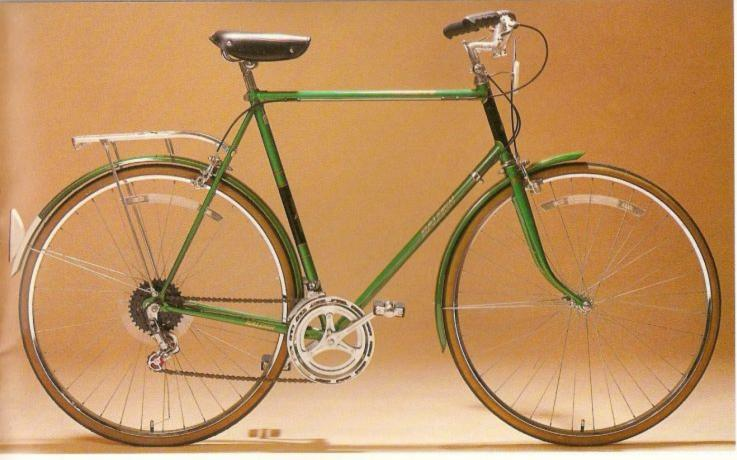
Frame: 3-Speed Sprite: Size: Gents: 21½", 23½", 25". Ladies Std.: 19½", 21½", 23". Constructed with Raleigh lightweight lugs & Raleigh 20-30 high carbon steel tube. Features brazed-on cable eyes & kickstand plate. 10-Speed Sprite: Size: Gents: 21½", 23½", 25". Ladies Mixte: 19½", 21½". Constructed with Raleigh lightweight lugs & Raleigh 20-30 high carbon steel tube. Features brazed-on steel tube.
