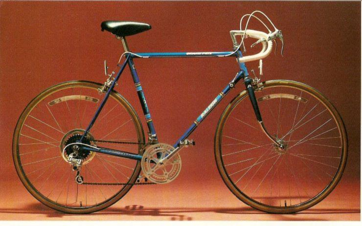
Frame: Size: Gents: 19%", 21½", 23½", 25½". Ladies Mixte: 19½", 21½". Constructed with Bocama feature cut lugs & Raleigh 20-30 high carbon steel tube. Features brazed-on cable eyes, guides, downtube stop & kickstand plate.
