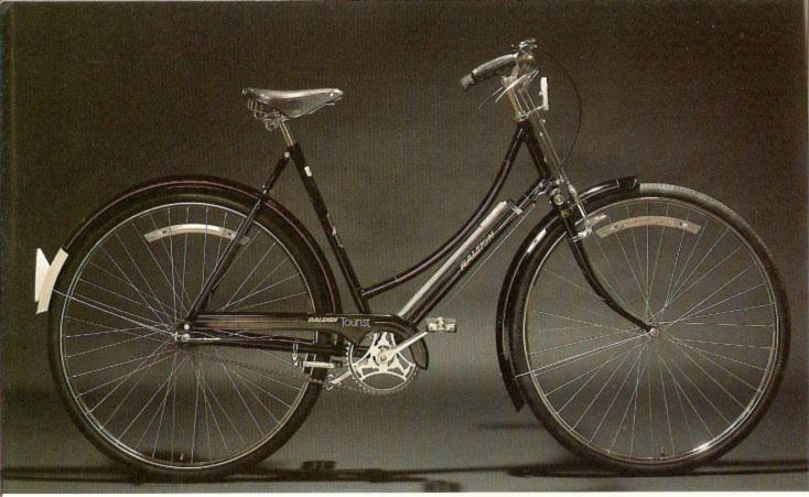
This rugged model is the only 28" wheel lightweight bicycle available in America with Raleigh quality. Designed and styled after the traditional London Bobbies bicycles to provide many carefree years of cycling pleasure. Features: the dependable Sturmey Archer AW 3-speed hub gear, traditional roller lever brakes (1), 28" x11/2" roadster tires for a smooth comfortable ride no matter what the road conditions (2), plus tire pump and saddle bag.
