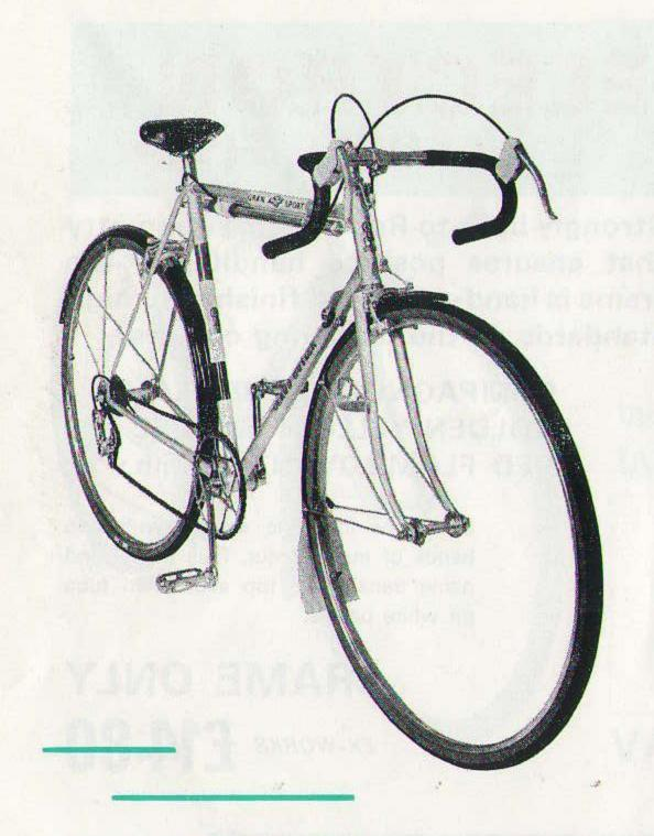
Designed for all types of general road use this machine is fitted with a Velox gear, the latest by Campagnolo with the well proven Valentino front changer on Ten Speed models. Centre-pull brakes provide extra stopping power —
