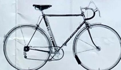
MODEL 84. FRAME : 21", 22", 23", 24", built with Reynolds 531 Tubing to upright angles. FORKS : Chrome plated — Oval pattern, fine taper, 531 blades. WHEELS : 27" x 1 1/4" Weinmann Alloy rims, large flange Hubs, double butted spokes. Dunlop Sprite tyres. HANDLEBARS : G.B. Alloy 15/16 dia. STEM : Alloy 2 1/2" forward. BRAKES : Weinmann 999 Centre Pull. SADDLE : Narrow Racing pattern. GEAR : Campagnolo or Huret Allvit Five Speed. Matching Mudguards and Accessories. FINISH : Purple Flamboyant.
