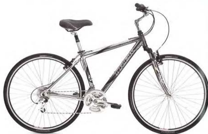
7200™ Frame Alpha Aluminum Front Suspension RST, 50mm Wheelset Alloy front, Shimano RM60 rear hub; Matrix 750 rims Crank Shimano TX71 48/38/28 w/chainring guard Rear Derailleur Shimano Alivio Colors Matte Cool Silver/Matte Wedgewood Blue; Black Chrome/Smooth Silver
