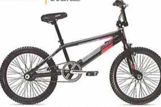
**FRAME:** Trek dirt design with an all-steel frame. Double-thick headtube and dropouts. **FORK:** Oversized 1-3/8" all-steel blades and superthick steer tube. **WHEELS:** Alloy rims with square knobby dirt tires for traction on all terrain. **COMPONENTS:** 175mm forged steel crank. Threadless stem system. Rear U-brake and front caliper brake. Trek steel pegs. **COLORS:** Blue or Black
