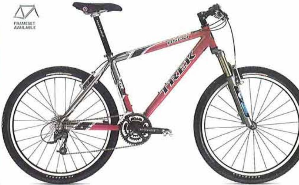
**FRAME** ZR 9000 Alloy™ is lighter than titanium and stronger than steel. Pro Race geometry transfers more power on climbs and descents. **WHEELS** Bontrager Race Tubeless are light but durable for years of off-road abuse. **SUSPENSION** Fox Float X fork (80mm travel) is tuned for XC racing.
