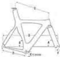
Front tube is measured from center of front tube top to center of seat tube.
