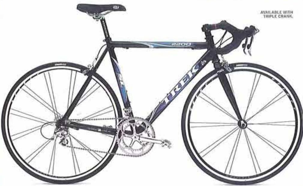
**FRAME** Alpha™ SL Aluminum. Superlight, large diameter tubing for exceptional durability and efficient power transfer. **FORK** Bontrager Race. OCLV Carbon design is light and fast. **WHEELS** Bontrager Select features Paired Spoke Technology™ for superior aerodynamics and lightweight strength. **COMPONENTS** Shimano Ultegra/105 9-speed shifting; Double or triple chaining. **SIZES** 50cm, 52cm, 54cm, 56cm, 58cm, 60cm **COLOR** Titania Black
