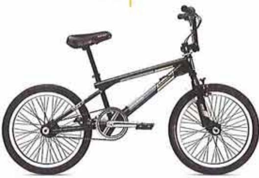
**FRAME:** Cro-Moly mainframe design. Trek Air geometry blends the best of vert and street bikes. **FORK:** All Cro-Moly with 1-1/8" blades. **WHEELS:** Tall alloy rims with freestyle tires for traction on all terrain. **COMPONENTS:** Trek tubular Cro-Moly crank. Threadless stem system. Front and rear U-brakes. Trek steel pegs. **COLOR:** Black
