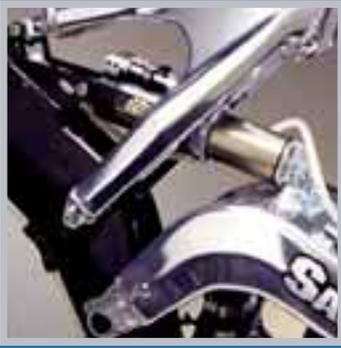
This is the heart of the San Andreas' distinctively smooth, yet responsive feel. The main frame, swingarm and subframe are all linked together at this pivotal (excuse the pun) point to yield the optimal suspension for the best ride of any monocoque suspension frame available!
