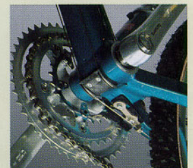
Klein's Chain Control Device™ keeps the chain from sucking between the chainring and chainstay by sweeping it clean and avoiding chain suck.
