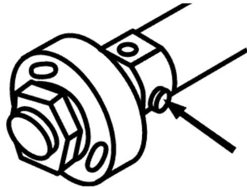
internal damping adjustment using set screw. Turn clockwise to increase compression damping. Turn counterclockwise to decrease compression damping. Standard setting is 4.5 turns out from fully closed.
