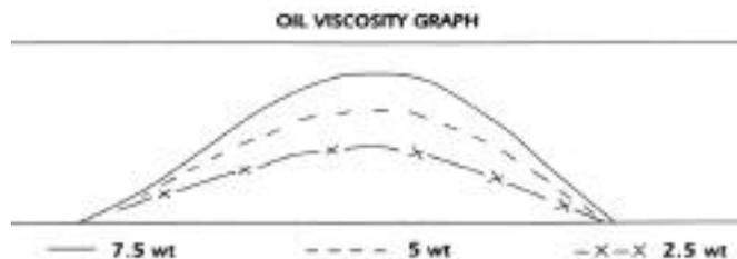
The heavier the fork oil weight, the more damping it will provide. 5-weight Maxima oil is stock in Manitou TPC and TPC Sport forks, but this oil viscosity can be increased or decreased in weight for differing riding conditions and styles
