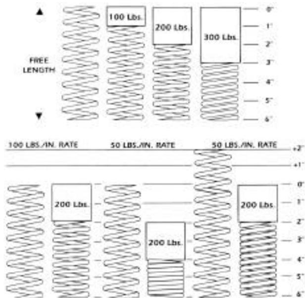
Fork spring compression is dependent on the weight placed on them, the length, and the progressivity on the spring
