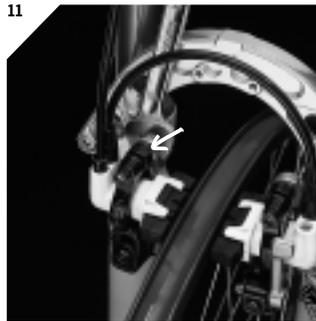
**11** Former MAGURA models came with a silver elbow. You need a 1.3mm open end wrench for correct adjustment (arrow). **The black and silver elbows are not inter-compatible!**
