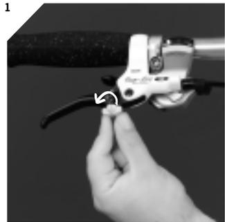
brake pad wear adjustment HS 33 models
