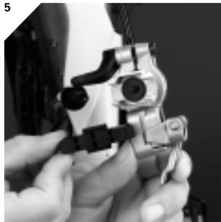
**5** To change the brake pads; open the quick release, remove the brake from the cantistud, pull out the old pad and then just snap in a new one. After removing the wheel, pull out the old pad and snap in a new one on the other side. That's all!
