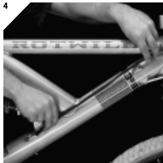
**4** Mount the hose installation kit for the rearbrake. Measure the distance between both cablestops. **Due to shrinkage, cut a length of heatshrink tube that is 10mm longer than the measured distance.**
