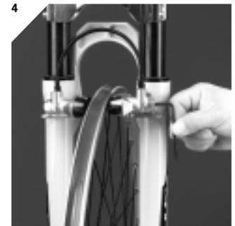
**4** With FIRM-tech you adjust the brake pad to the rim on both sides with the 5mm allen screw. **Shorten the hose and pad wear adjustment as described in the respective chapters!**
