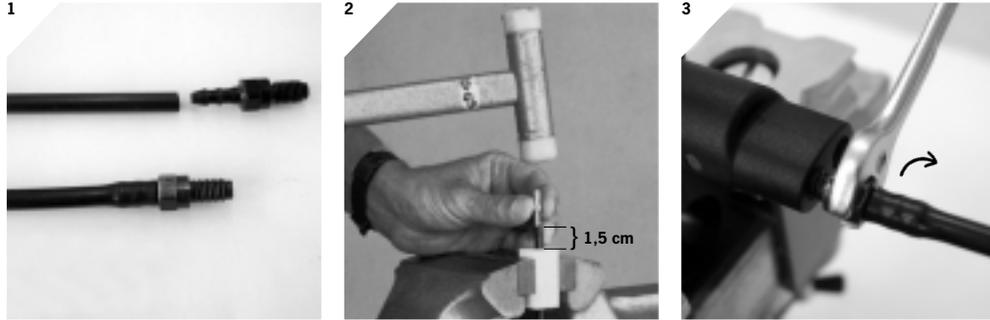
**1** Repair of a HS 11 main hose with barbed adaptor connection.
