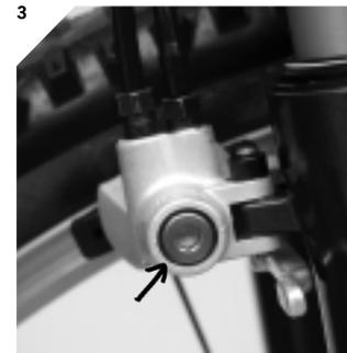
**3** Adjust the brake pads to the rim width with the 5mm allen screw which is integrated in the brake cylinder. By turning the screw clockwise the pad approaches to the rim.
