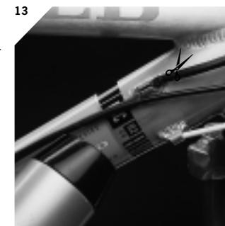
**13** Use an extra piece of heatshrink tube which you slide over the exposed end of the carrier cable. Shrink the heatshrink tube over its entire length with a hairdryer. **Only use a hairdryer! Never use a lighter or a heatgun. Protect your frame and decals with carton before.**
