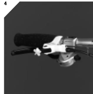
**4** Turn the brake lever (HS 33/11) horizontal on the handlebar so that the bleed bolt is at the highest position. Turn back **fully** the TPA knob or allen adjustment bolt in the brake lever. Remove the bleed screw in the brake lever.
