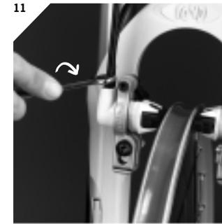
**11** Do not crossthread! After initial start by hand use an 8mm open end wrench. **(Tightening torque 4Nm/34 in.lbs).**
