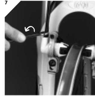
**7** Unscrew the 8mm sleeve nut at the slave cylinder and pull out the hose **carefully**. **Never activate the lever blade with the system open! Hold the tubing carefully in order to avoid any loss of oil!**
