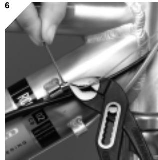
**6** Slide the adjustable barrel over the cable and pull the cable **firmly** through the other cablestop with pliers. Push, with the pliers, the adjustable barrel against the cablestop and tighten the 2mm bolt with an allen key. Cut off the remaining cable so that it is flush with the barrel.
