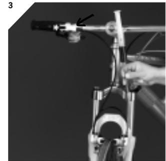
**3** - Put the filler tube on the syringe and fill **completely** with MAGURA BLOOD mineral oil. In the case of an emergency, cooking oil will work, but needs to be flushed out after the return to civilization. **Never use DOT brake liquid! Pay close attention not to have any air in the tube or syringe.**
