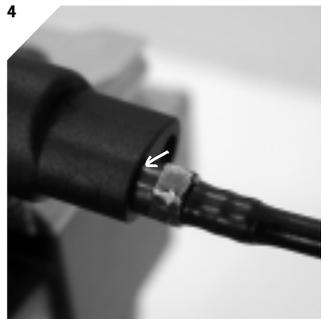
**4** Correctly installed repaired hose on an HS 11. The barbed fitting is **flush** with the brake lever (arrow). The brake now has to be re-filled as described in the chapter 'filling and bleeding'.
