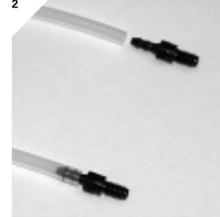
**2** Push (by hand) a barbed fitting into **both** the transparent filler and vent tubes.
