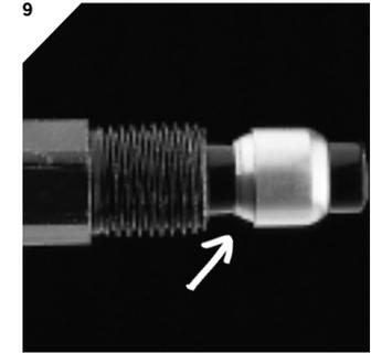
**9** Slide the sleeve nut and a **new** olive on the hose. **When you use old, brass colored olives, the grooved side (arrow) points toward the sleeve nut.**
