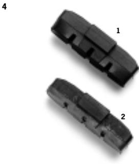
**4** New (1) and worn (2) brake pad. When your brake pads are worn as shown it is time to change them.
