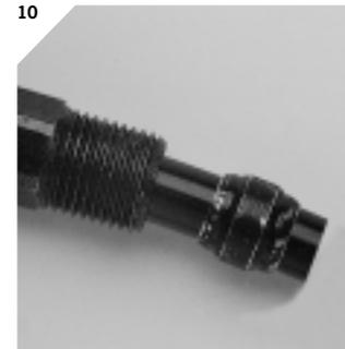
**10** The black olive cannot be mounted incorrectly, as it is symmetrical. Push the hose **all the way** into the slave cylinder.
