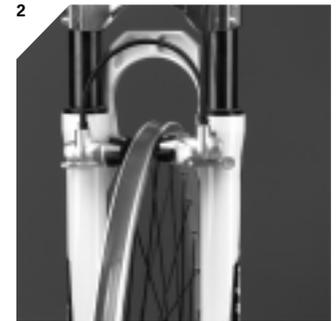
**2** Close the quick release: Push the brake cylinder back towards the fork. Close the quick release by doing the same. That's all! **A booster is not necessary with FIRM-tech and not foreseen either. It is not possible to mount one!**
