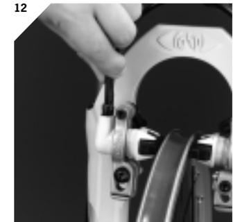
**12** Always check for correct installation by pulling on the hose. **Make sure that the system has no leaks by activating the levers and checking all connections.**
