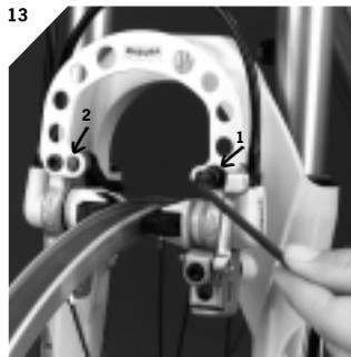
**13** Installation of a brake booster. The side with the single wide hole is mounted on the quick release side of the adaptor. Do not forget the washer under the head of the fitting bolt (arrow 1). **(Tightening torque 4Nm/34 in.lbs)**. On the opposite side one of the round holes just slips over the existing bolt. If ever your tyre should touch the booster here (arrow 2) just cut it off with a wire-cutter.
