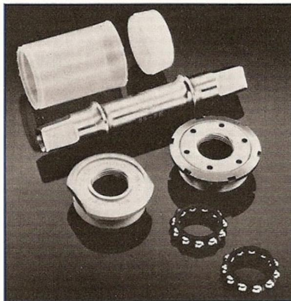
The bottom bracket is similar to other Campagnolo bottom brackets. The symmetrical axle is case-hardened steel. Both axle and cups are precision ground and rotary polished for use with Campagnolo high precision bearings.
