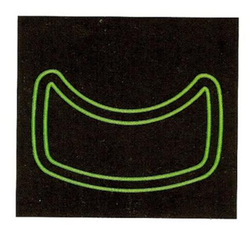
The cross-section design for clincher tire rims is just as important as it is for tubular rims with the additional consideration of the rim's ability to hold the tire bead at pressure above 100 PSI.
