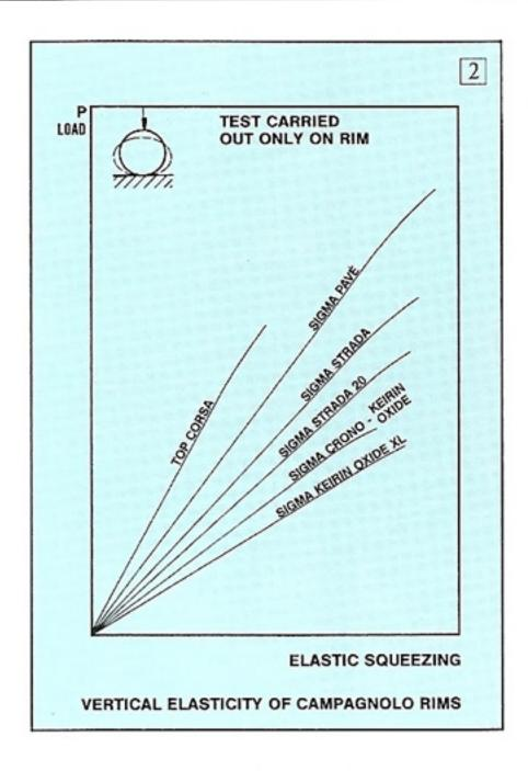
compression. The rest of the system does not undergo important alteration. On the basis of these considerations, Campagnolo has worked out profiles and materials for its whole range of rims that solve both problems: resistance to vertical loads, and comfort for the racer.
