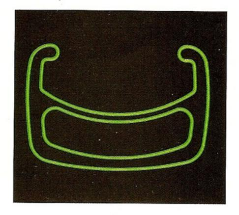
Computer design coupled with wind tunnel testing has enabled Campagnolo to design an aerodynamic rim whose profile («V Profile») prevents the breakaway of air flow (turbulance). In comparison to a rim with a normal cross-section the special sidewall camber of this Campagnolo's rim substantially reduces the effort required to penetrate air.
