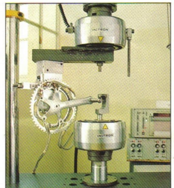
rings, from 39 to 57, is available. These are made by pressing. They are manufactured in very resistant light alloy used in aeronautic applications, which guarantees that they will last a very long time.
