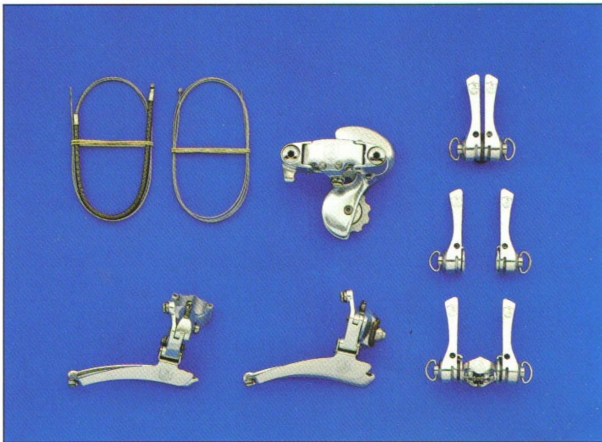
the friction and play of the roller may be adjusted by means of the dust caps. The play of the roller can thus be adjusted, varying with the tension of the chain, to ensure smooth running of the chain on every occasion, thus precious hundredths of a second are gained to those who do not use professional equipment.
